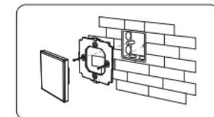
Fix the base on the bottom case with screw.
