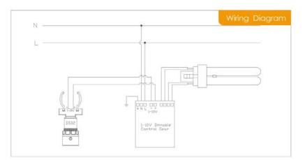
NOTE: Please be noted that whether or not the lamp can be switched off depends on the control gear. DS02 has the lowest voltage output 1.1-1.2v, if control gear can switch lamp off at this voltage, the lamp can be switched off. Hytronik also supplies a 1-10v dimmable 25W LED driver which can be working with DS02 to switch off lamp if needed.
