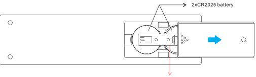
Note:Before the first use, please remove the protective film on the battery.
